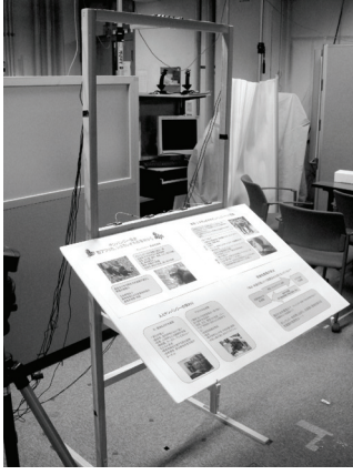
Figure 2: Poster presentation frame. Microphone arrays are set at the top of the frame.
