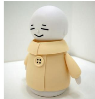
Figure 1. Bono Bot, the group conversation facilitation robot.
