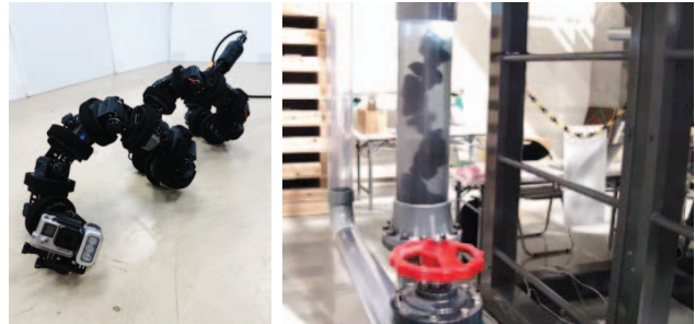
(a) 2-m in-pipe snake robot (b) Snake robot climbing a vertical pipeline Fig. 1. In-pipe snake robot used in this paper.
