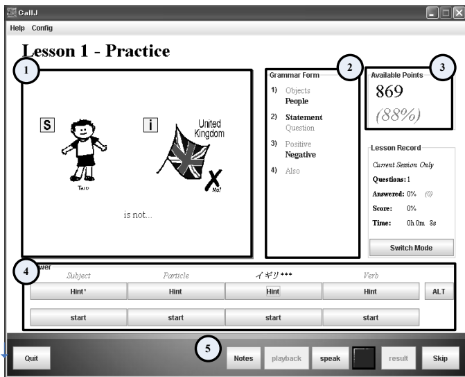
Fig. 4. Screen shot of CALLJ; 1: Concept diagram, 2: Desired form guide, 3: Score, 4: Answer area and hint display, 5: Control button panel
