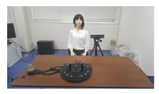
Figure 1: The setup of ERICA's demonstration system, with microphone array and Kinect sensor.
