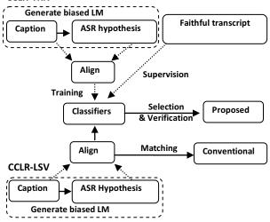
Fig. 1 Framework of proposed data selection for lightly supervised training.
